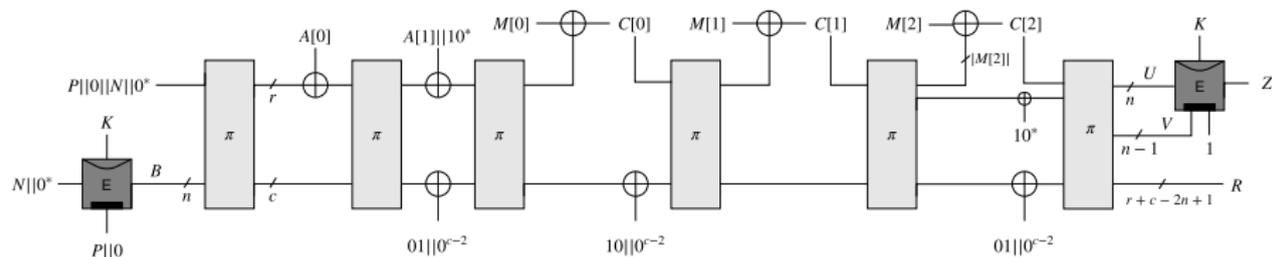
ciphertext  $(C[0]C[1]C[2], Z) = \text{Enc}_K^P(N, A[0]A[1], M[0]M[1]M[2])$
