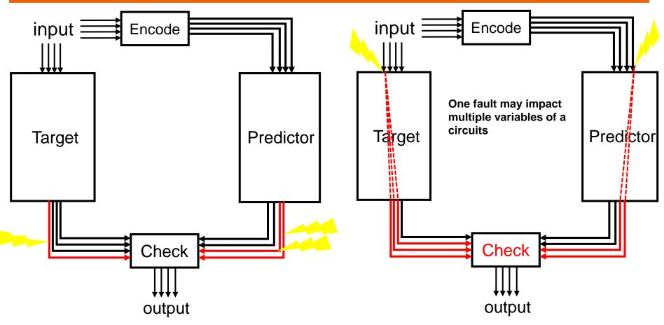
Basic Structure of code-based concurrent error detection schemes
